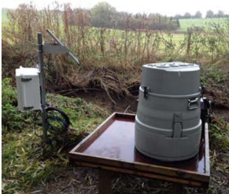
Figure 13. Automated water sampling equipment is installed at the downstream end of each stream catchment. We are using this equipment to near-continuously monitor nutrient and sediment concentrations. In the autumn when surface runoff and drainflow normally restarts, we are using this equipment to collect samples for pesticide analysis. The photograph shows an Isco sampler on the right with a solar powered data logger .
